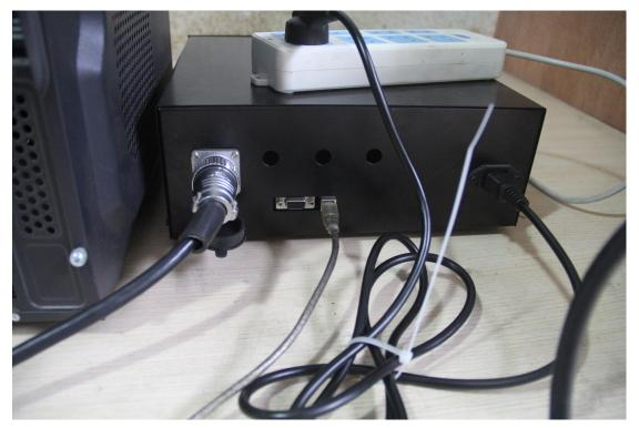
A: controller power line interface (need to ground wire, otherwise long term use will cause harm to display)
